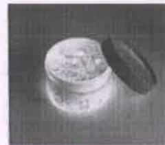
'Mr Frosty' Used to freeze cells
